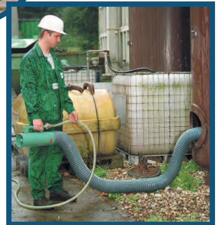
8 1620 0010 Pneumatic Air Mover, 7" dia. 2366 cfm output @ 90 psi
