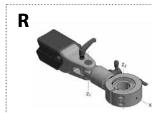
X:Turns 360°. 64 Lockable positions Z1:Turns 90° left. 5 Lockable positions Z2:Turns 360°. 8 Lockable positions
