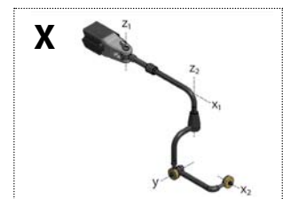
X1:Turns 360°. Lockable each 45° X2:Turns 360° Y:Turns 360° Z1:Turns 90° right & left. Z2:Turns 360°
